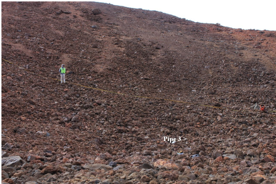
Figure 4. Extent of current permafrost along an approximately east-west oriented ERT survey line. A person to the east (32m along the survey line) and a red backpack to the west (16m along the survey line) mark the boundaries of the permafrost body. "Pipe 3" is visible in the foreground.
